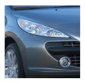
The 207 CC GT 1.6 Turbo benefits from elliptical module H7 headlamps with static directional lighting. This system consists of two additional lights mounted in the main headlamps which light independently of each other at the request of an electronic control unit (ECU). The latter triggers lighting when the steering wheel angle records the value of 25° to 50°, depending on vehicle speed, allowing better lighting of the inside of corners.
