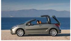
Developed from the 206 CC, the operation of the 207 CC roof differs significantly in terms of convenience, thanks to its entirely automatic operation without the need for any manual roof release. The only manual operation consists of pressing the control button for around 25 seconds during which time the opening or closing cycle is completed after all four windows have been lowered automatically.
